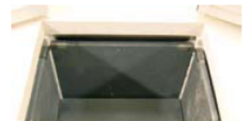
Furnace chamber of S 73/HS with SiC-plates as muffle function
