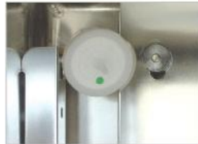
Gas supply line filter
