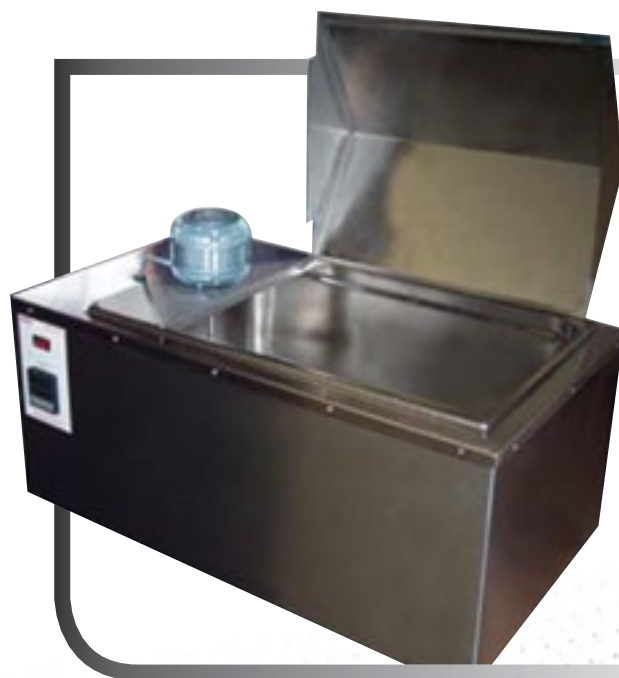
Water Bath with top mounted stirrer and optional stainless steel hinged lid shown above.
